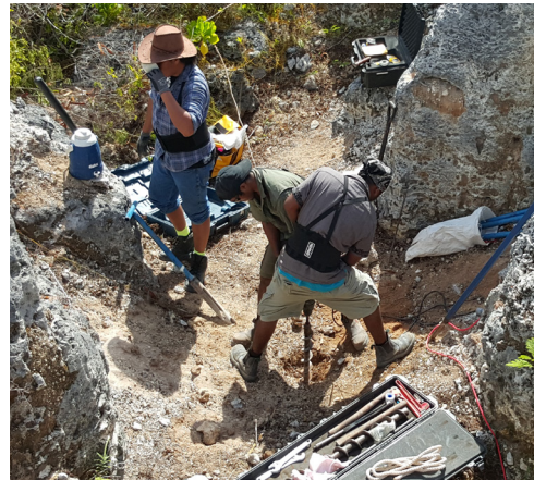
Ronphos field team conducting the first series of drilling to test the depth and quality of phosphate
